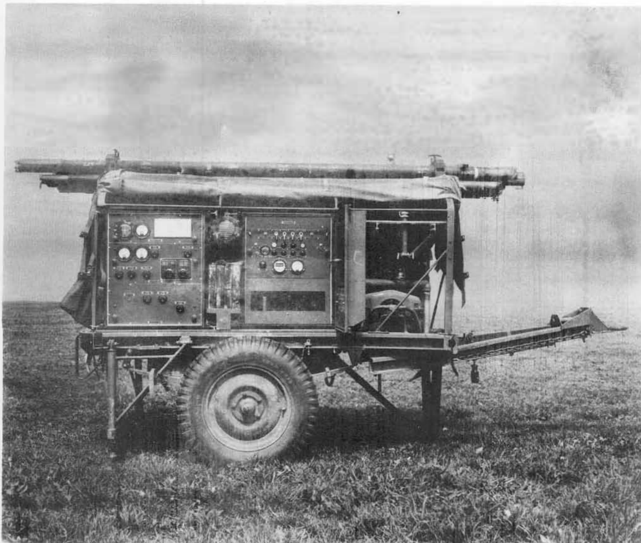
Radio Set AN/CRN-2 packs into a simple trailer which permits rapid transport by air or ground.
