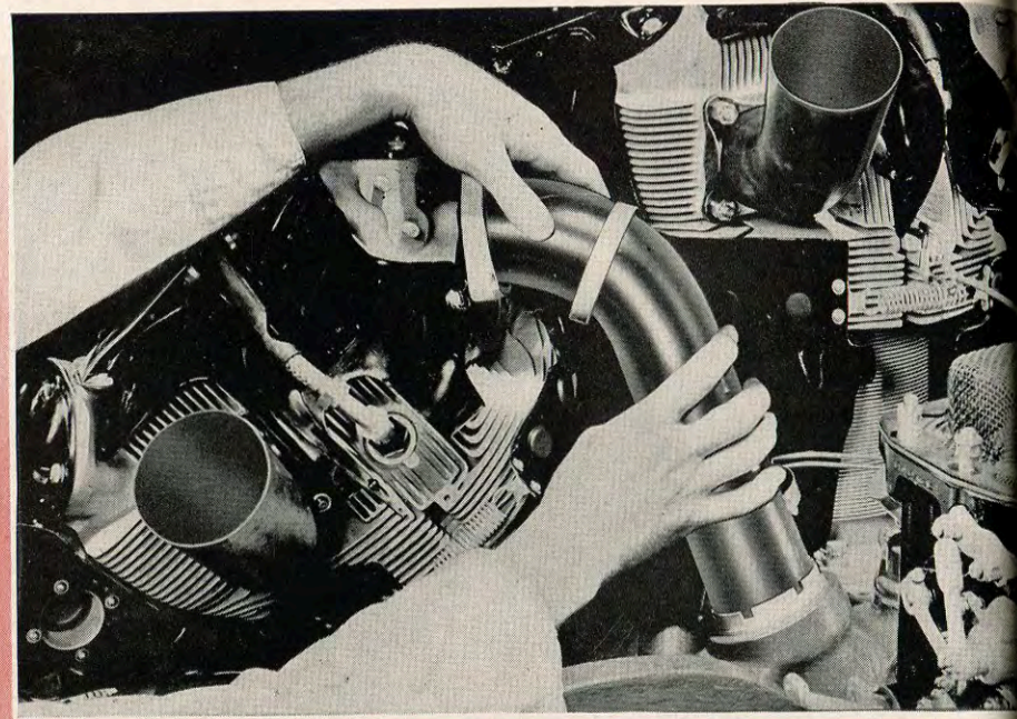
INSTALL INTAKE PIPE
