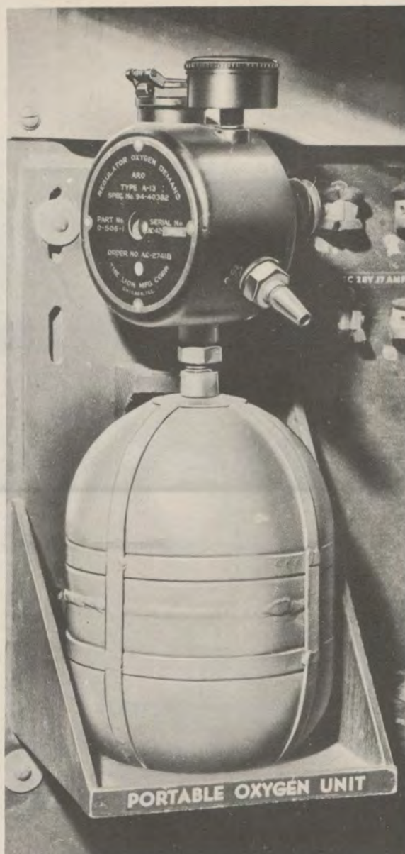
A-4 walk-around bottle on bracket at airplane station
