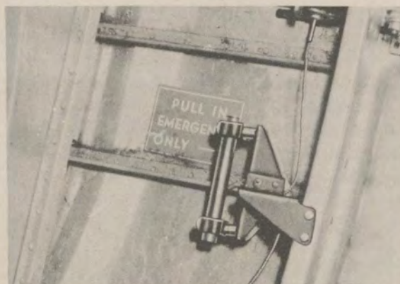
Emergency Release: Tail Gunner's Hatch
