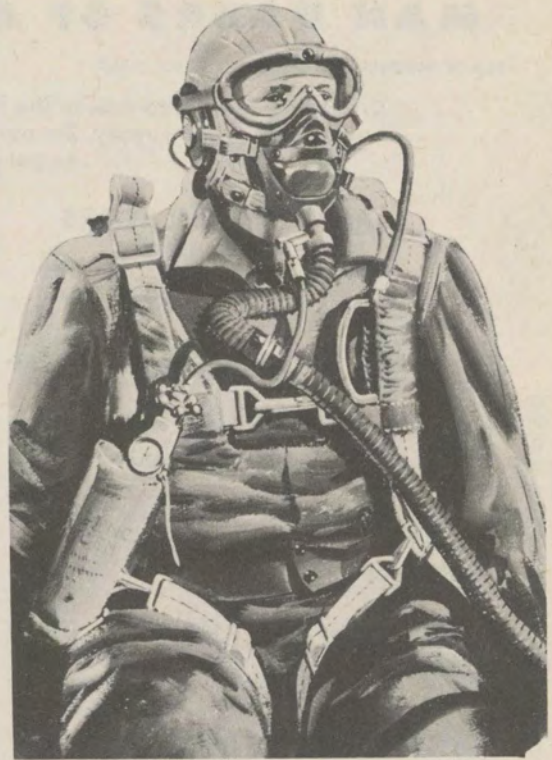
Keep bailout cylinder hose plugged into mask
