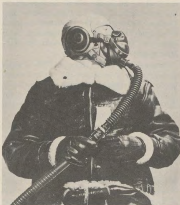
Clip hose in position to allow full head movement
